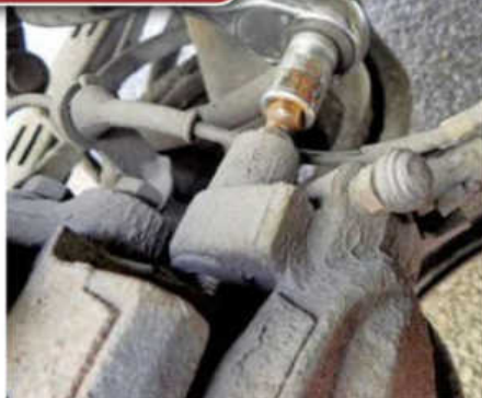
2 As with the front brakes, use a 5mm Allen key to remove both caliper slider pins. These fit into the rubber sleeves – if they are tight, the caliper can stick. On reassembly they are torqued to 28Nm, both front and rear – do NOT overtighten!
