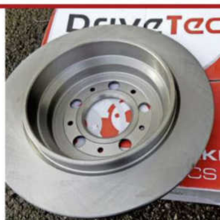
3 Autosessive supplied the new DriveTec discs. They come in either 'dry' form with a light grey coating that must NOT be removed (it's there to bed in the pads) or, in this case, coated in protective grease, which needs to be cleaned off with an aerosol brake cleaner.
