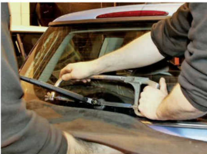
21 More trouble arose when we tried to detach the wiper arm from the spindle on the replacement tailgate. It had seized, so we had to hacksaw through it so we could remove the motor.
