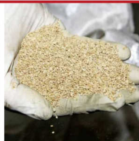
2 The blast medium is crushed walnut shells. They are considerably less abrasive than conventional beads, used for shot blasting, so they will remove carbon without damaging soft aluminium castings.
