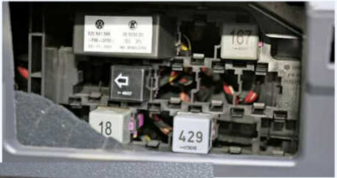
14 This fusebox assembly, with the car's diagnostic socket located at its centre, is located under the fascia on the right-hand side. It is normally hidden by a plastic cover panel, which has been removed for this photo to be taken.
