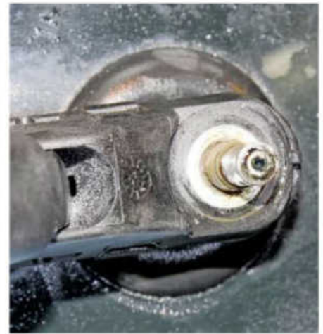
20 With the wiring in position, we tested the wiper. Sadly, the end of the washer jet had snapped off, so it wouldn't spray water over the rear glass. This is part of the motor, so we decided to reuse the one on our original tailgate.
