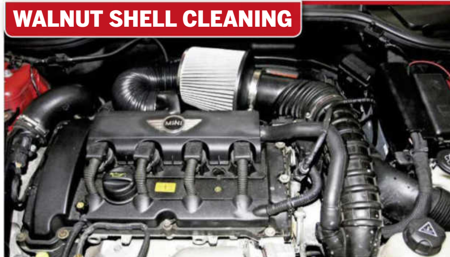
1 The French direct-injection petrol engine, used in MINIs from 2006, as well as various Citroëns and Peugeots, is particularly prone to inlet valve deposits.
