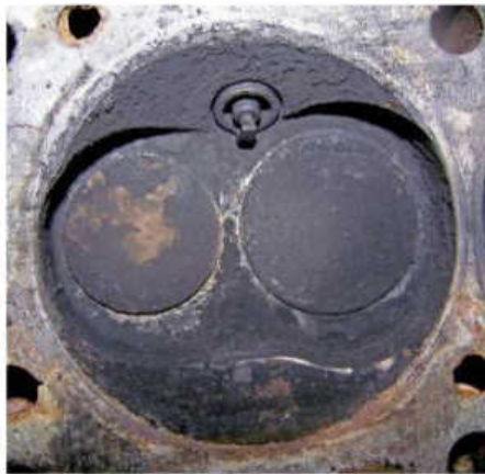
Carbon build-up within the cylinder can ignite the fuel/air mixture at the wrong moment, resulting in poor running and, possibly, damage to the engine.
