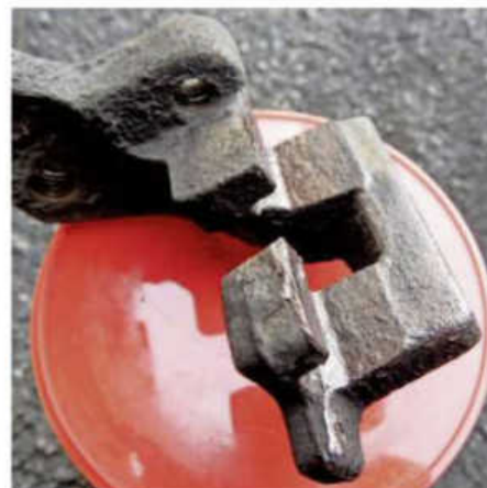
6 Before refitting, the caliper brackets need to be cleaned. A wire brush will get things started, and, if required, use a coarse flat file to clean the areas where the pads fit back to bright metal, before smearing lightly with copper grease.
