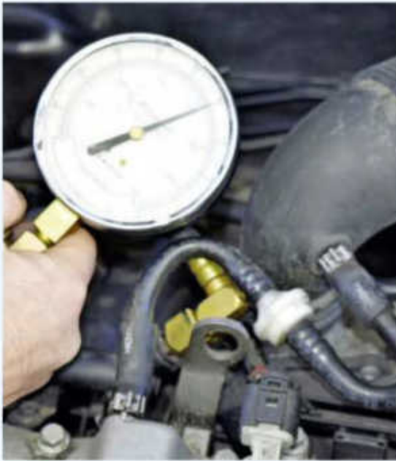
12 The fuel pressure can be assessed by connecting a pressure gauge via the Schrader valve at the left-hand end of the fuel supply pipe for the injectors. Before running the engine, ensure that all connections are tight, to avoid fuel leaks.
