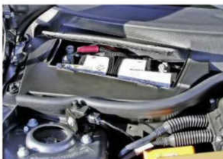
A prototype BMW MINI E electric car from 2008, used a 12-volt battery to power the heater and the on-board electrical system.
