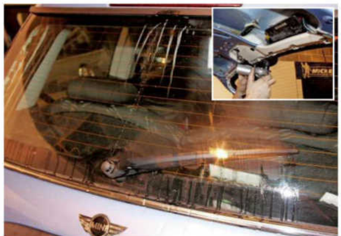
22 We had similar trouble releasing the wiper arm from our old motor, snapping off the end of the arm, but we managed to make one good rear wiper and arm out of two. After fitting our old wiper motor, we tested it and the screenwash sprayed out.
