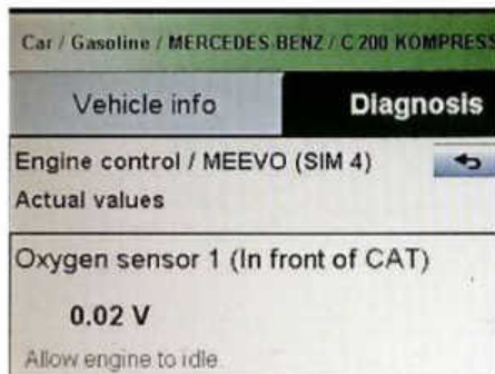
These are live data readings showing the Lambda probe signal voltage.
