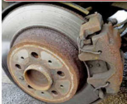
1 The rear discs mirror those on the front with the 10mm retaining bolt. The handbrake shoes are inside the centre brake disc 'bell'. Notice how the ends of the anti-rattle spring locate behind the 'ears' on the caliper itself. Ours had been fitted incorrectly.
