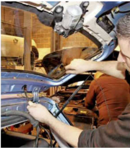
18 We fed a thick length of wire through the top section of the tailgate, attaching it to the respective end of the wiring loom and pulling the two back through. This helped on the offside, where space is tight.
