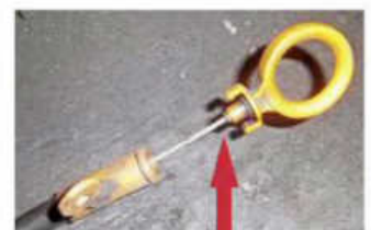
The top guide of the Audi A3's dipstick had broken away.
