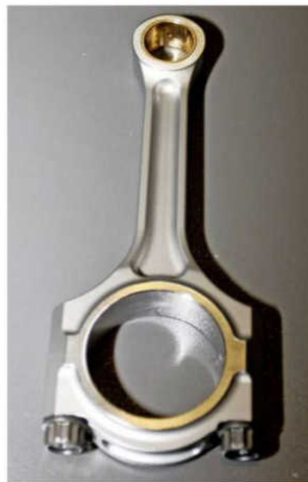
As a result of shortening the piston, the connecting rods were extended by 9%.
