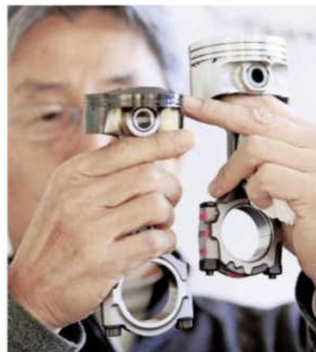
The pistons had to be redesigned completely. The new, shorter pistons reduce weight by 40% and their inertial mass by 30%.
