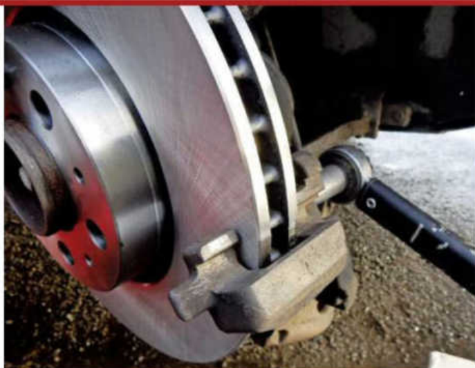
10 Fit the new brake disc to the cleaned and copper greased hub and do up the 10mm retaining bolt (10Nm) before fitting the cleaned up caliper bracket. For the best results degrease the disc and paint the inner 'bell' area with Hammerite so it doesn't get rusty.
