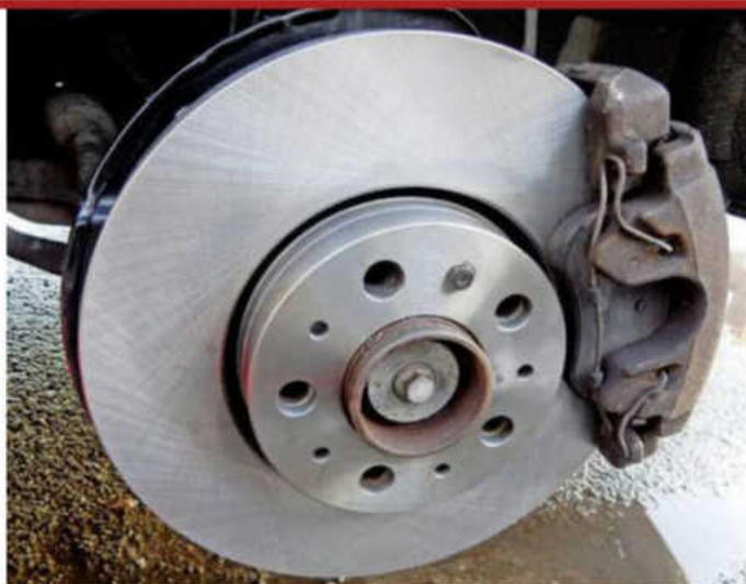
11 Looking much better than before. The new brake pad end 'ears' were lightly coated in brake grease and are now good for thousands more miles. More importantly, the car now brakes quietly and smoothly – the wobble has totally vanished.
