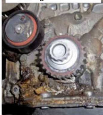
The coolant stain showed it had been leaking for some time.
